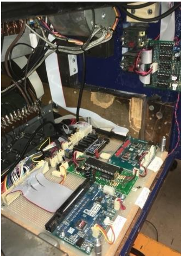
Fig. 89, 90 and 91 Pictures of the 'transformation B3' to the Modular Hammond. Installation of MIDI on keys and drawbars, painting of the cabinet, installation of electronics.
